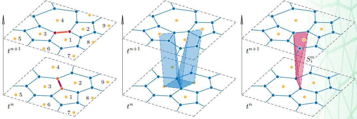
Figure 2: Space time connectivity with topology changes, degenerate sub-space-time control volumes and crazy sliver element.
