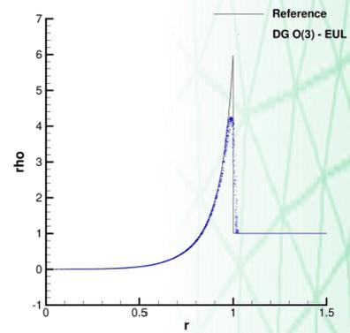
Figure 5: Sedov explosion problem solved with our third order ALE-DG scheme. The topology changes maintain a high quality mesh and the Lagrangian framework (middle) allows to obtain a scatter profile perfectly in agreement with the reference solution and much better than what obtainable with an Eulerian scheme (right) of the same order. Note that our a posteriori FV limiter activates exactly only at the shock location (blue cells in the left panel).
